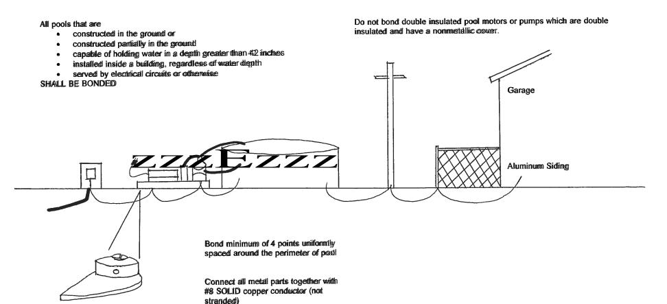
Use stainless steel, brass, copper, or copper alloy, lugs and hardware
